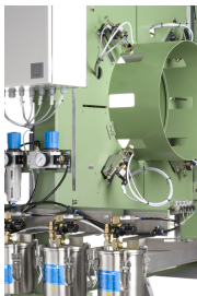
COLOR MARKING SYSTEM Precision marking of defects on the test piece
