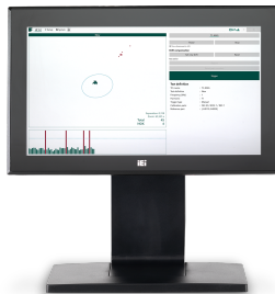
PANEL PC FOR TCL High-performance Industrial PC with touchscreen for eddy current testing
