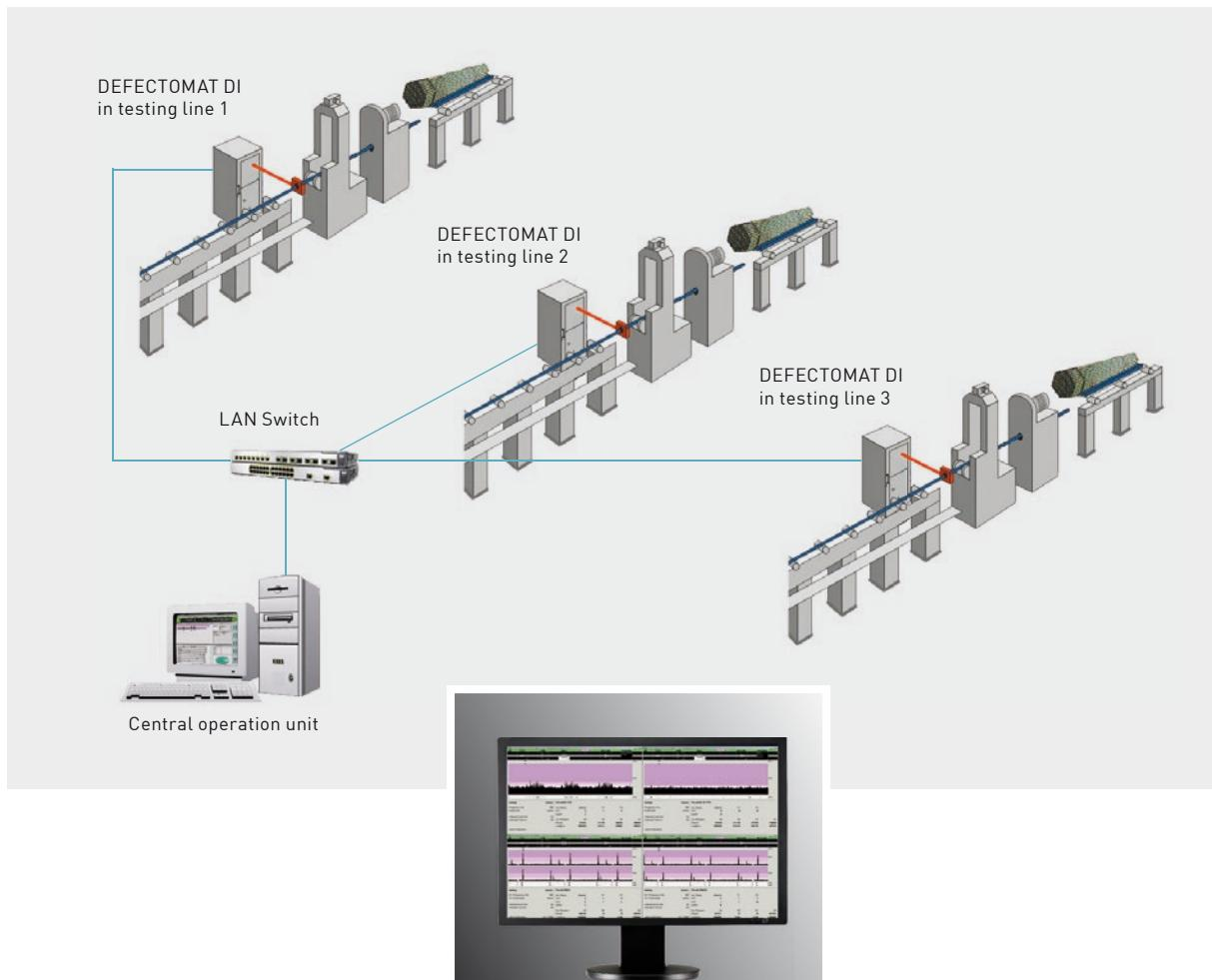
The DEFECTOMAT DI integrates all necessary functions and interfaces for eddy-current testing, and permits the connection of maximum two test coils or probes. The compact dimensions of the DEFECTOMAT DI allow close integration to the testing line.
