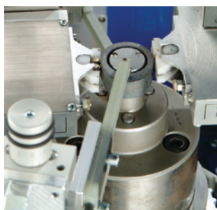
Figure 2: Crack detection on cams with two testing probes on the contact surface and one testing probe on each face side
