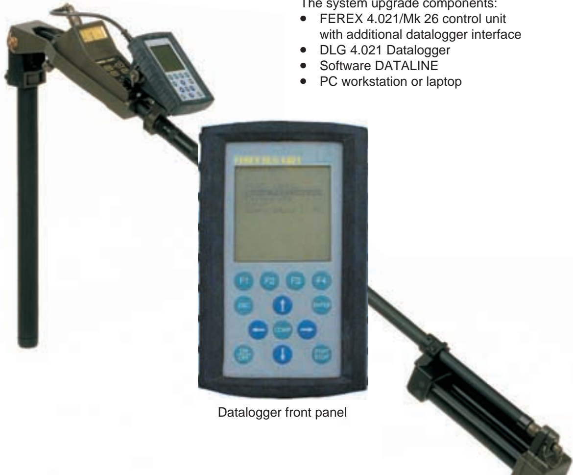
Fig. 15 FEREX 4.021/Mk 26 Land Search Configuration with Datalogger DLG 4.021
