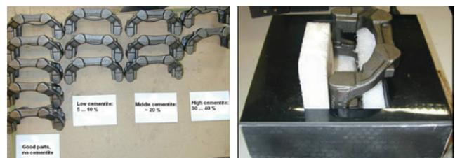
Fig. 2: Cast components and bracket in the test coil
