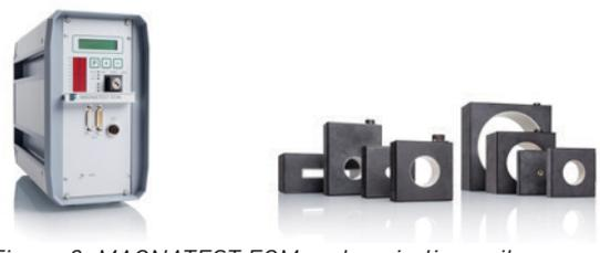
Figure 3: MAGNATEST ECM and encircling coils
