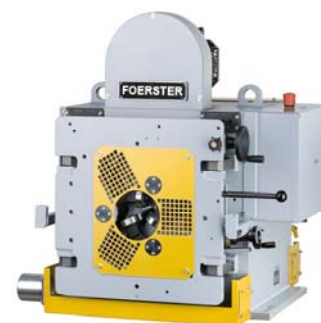
Fig 1: CIRCOFLUX sensor system
